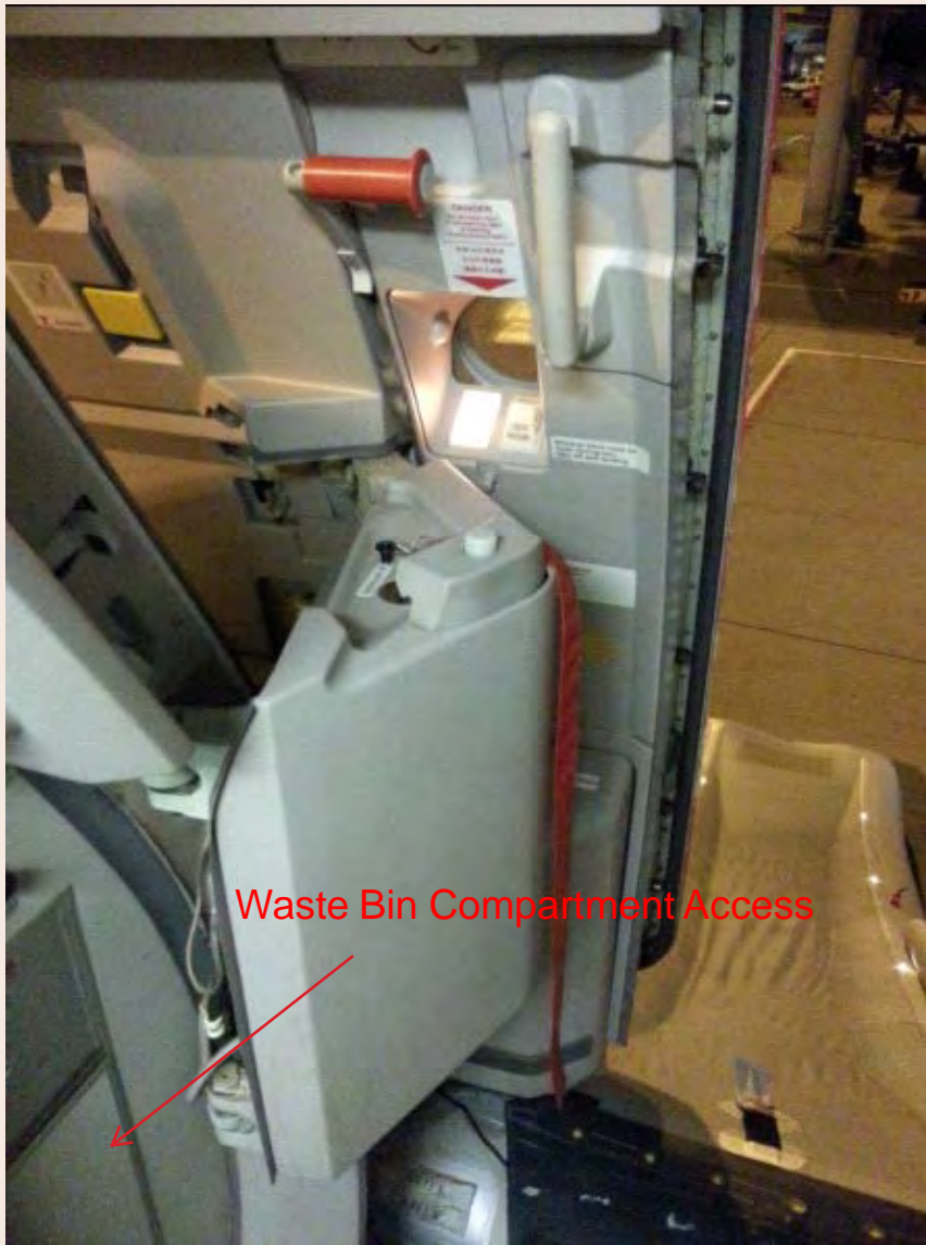
Cleaning supervisor opened the R1 door from inside while the door was armed which resulted in the inflation of evacuation slide
